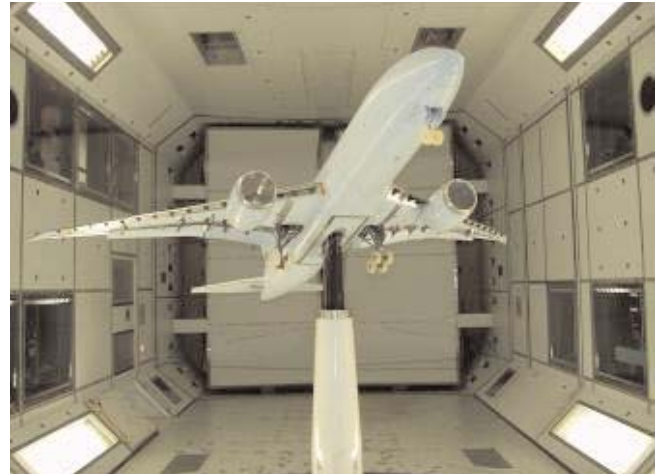
Model in the test section of the QinetiQ 5m Wind Tunnel
