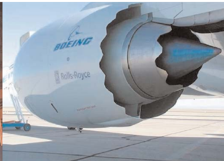
Serrated nozzle developments on the engine and in the NTF - Pictures courtesy of Boeing and Rolls-Royce
