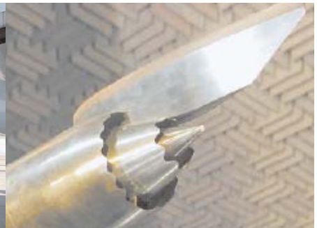
Serrated nozzle developments on the engine and in the NTF - Pictures courtesy of Boeing and Rolls-Royce
