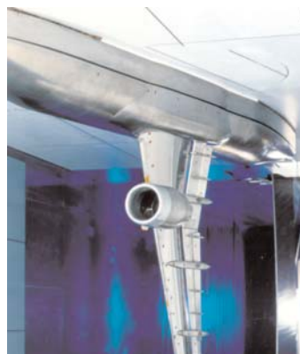
Half Model in High Lift Configuration in the Test Section
