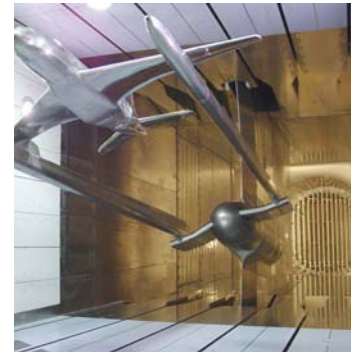
Aircraft model on the Twin Sting Rig in the Test Section
